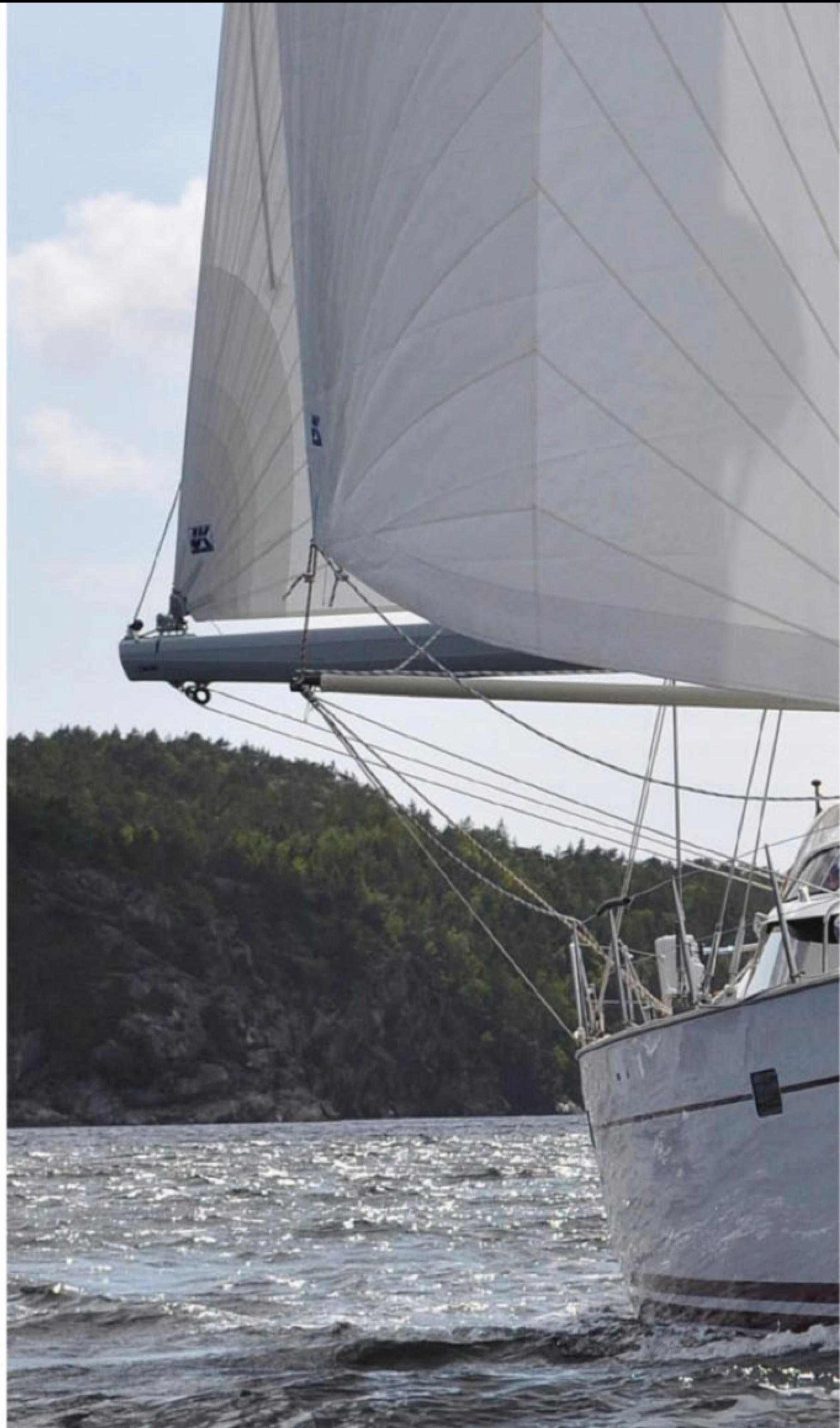
▲ Above: The Simbo rig in action with whiskerpoles and twin headsails set.
